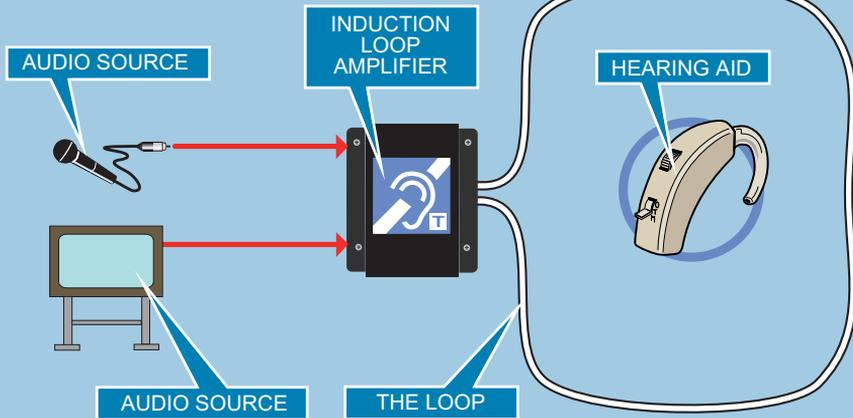
Some induction loop systems may require additional audio sources such as multiple microphone or line level inputs. To facilitate this, many PDA range amplifiers include a patented 'Outreach' socket which allows the connection of multiple inputs via a range of specially designed single gang audio connector plates. This system is described in detail on page 26.
