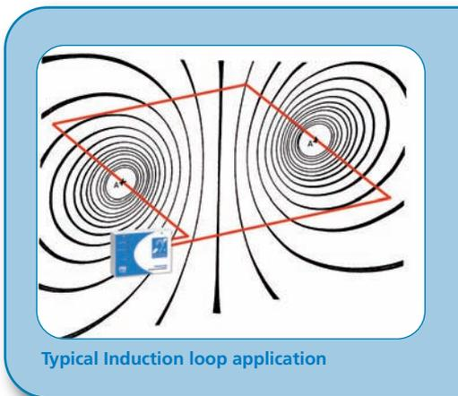
up by an unauthorised person in a neighbouring room, this is more concerning. BS 7594 suggests several technically complex solutions to prevent overspill that are reasonably effective. In many cases overspill can be reduced nearly as effectively and for much less cost, using the special loop patterns described below.
