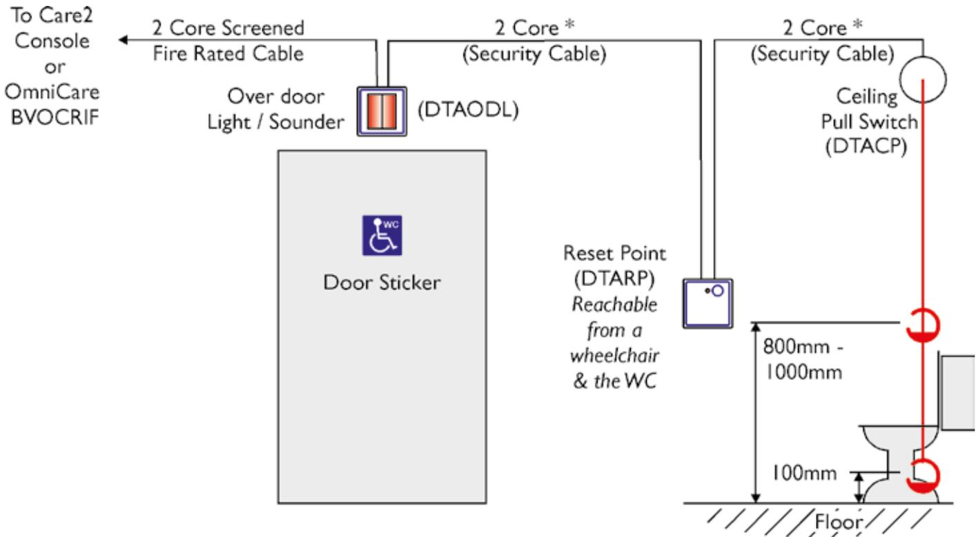
\* The Safety Earth connection **MUST** be fitted if Stainless Steel front panels or metal back boxes are used.
