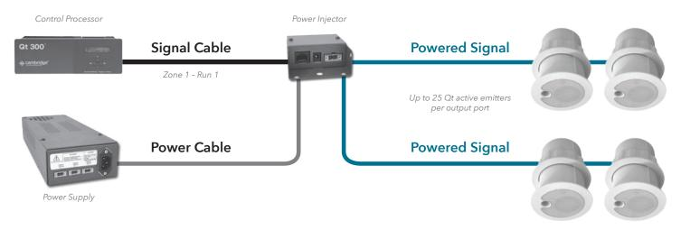
Signal Cable - Cat 3, 5, 5e, 6 UTP Category - Plenum Rated Cable Power Cable - 14/2 Plenum Rated Cable (ships with Qt Active Emitter Power Supply) Powered Signal Cable - Cat 3, 5, 5e, 6 UTP Category - Plenum Rated Cable (Active Emitters ship with 16 foot cables)
