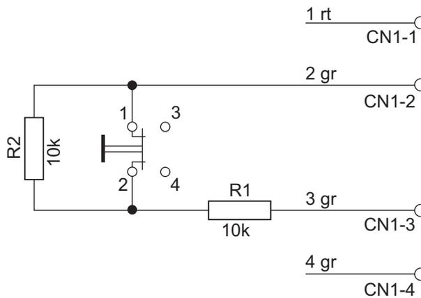
Fig. 1: Connecting the key switch as normally closed contact (NCC) for key lock function
