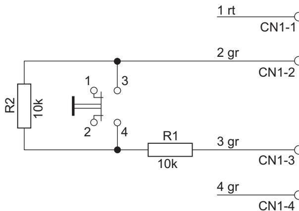
Fig. 2: Connecting the key switch as normally open contact (NOC) for special purposes
