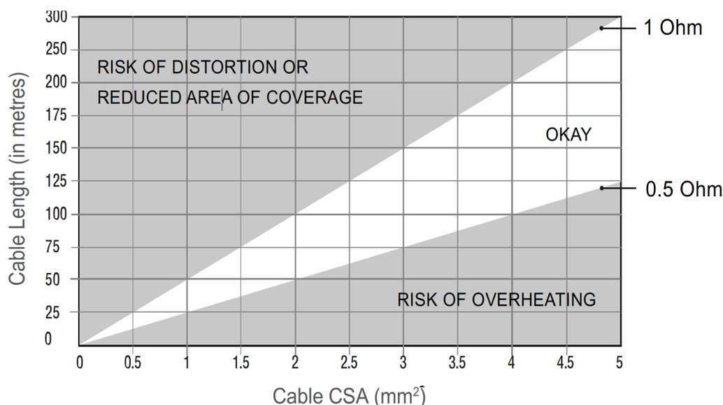
For example, to cover a room 15m x 10m (150m<sup>2</sup>) the loop cable would need to be 50m long (2 sides @ 15m and 2 sides @ 10m). The recommended cable CSA for a loop this length is between 1mm<sup>2</sup> and 2mm<sup>2</sup>. Therefore, an amp which can cover areas of at least 150m<sup>2</sup> using 1.5mm<sup>2</sup> cable would be ideal.
