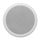
The CM20T two-way built-in loudspeaker can be used as a 16 ohms or 100 volt loudspeaker. In 16 ohms use, you can connect up to 4 loudspeakers in parallel on each channel of a standard 4 ohms amplifier. For 100 volt use, the CM20T is equipped with a high-quality 20 watts 100 volt transformer with several power tappings (20-10-5-2.5 watts). Therefore it can be used in projects with high ceilings or places with background noise where a little more power is needed.
