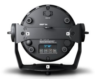
In order to effectively use the tilt function with the tilt screw when using as an uplight, and to achieve a more inconspicuous look, you must use a suitable tool to remove the mounting bracket by releasing the four T20 Torx screws (B) that secure the mounting bracket to the spotlight housing.
