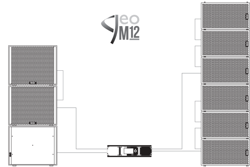
NXAMP4X4 Mk2 powering 3 X MSUB18 (one in cardio mode) and 6 X GEO M12
