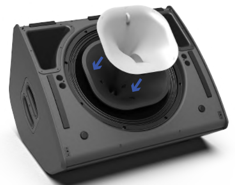
Grille removed, an additional magnetic flange can be quickly fitted to change directivity from 60°x60° to Asymmetrical
