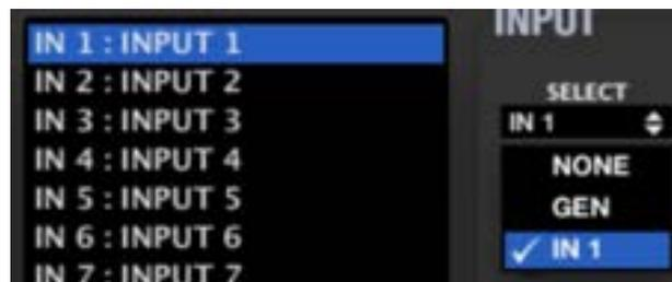
That means: INPUT 1 in the matrix processing can just take its signal from the internal generator or the audio source physically connected to IN1 back panel terminals. The same happens with INPUT 2 -> IN2, INPUT 3 -> IN3, ..... INPUT 9 -> DIN1, INPUT 10 -> DIN2, etc. (Digital inputs can be Dante or AES67)
