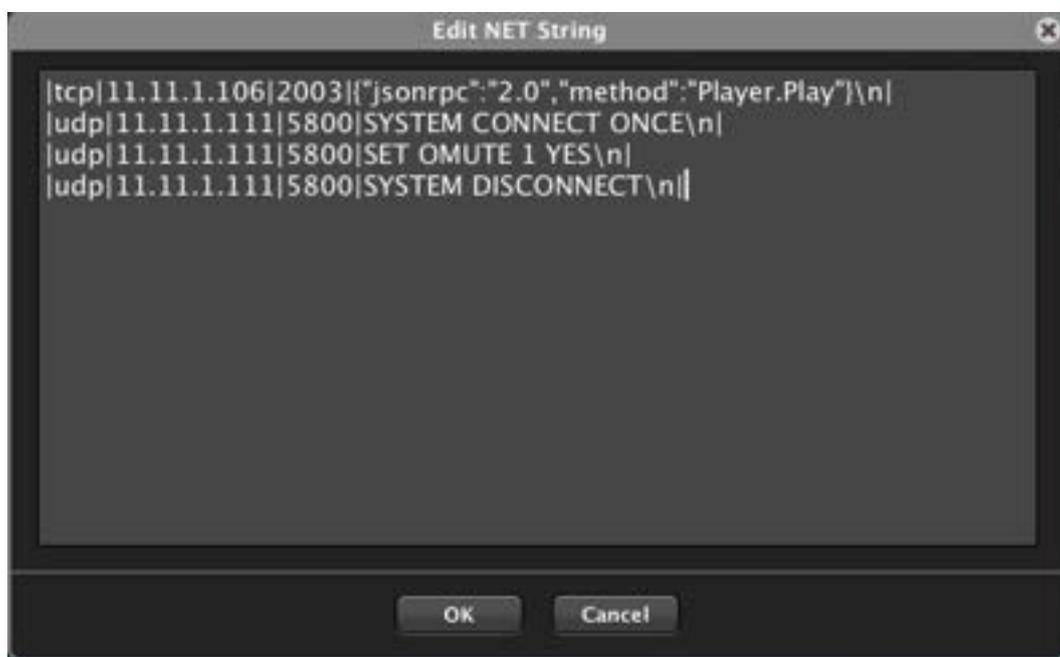
It is possible to send more than just one text string to different destinations. To do so, repeat the above specified format text the times needed. Now it’s possible to add carriage return (multiline text field) to visually differentiate the different messages to be sent.
