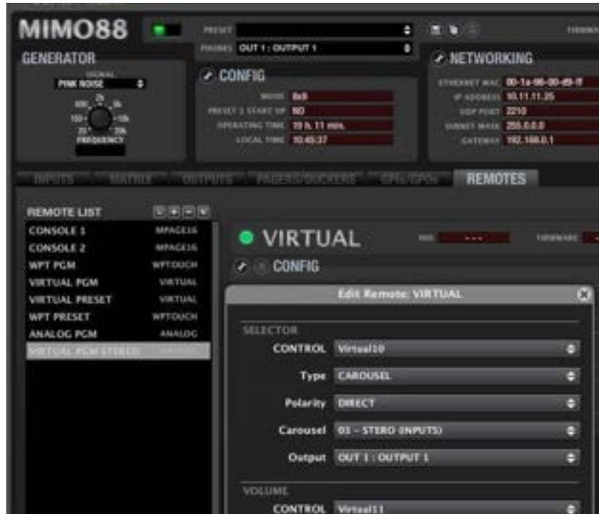
The virtual selector from the previous image, created in the REMOTES section of a MIMO88, can now be remotely controlled from a UCP:
