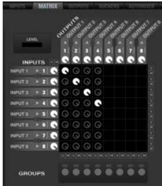
The image shows that the MIMO88CONF has the ability to process any mix of inputs you may have sent to one of the first 4 outputs on the unit. In other words, it is possible to generate up to 4 independent mixes, using any combination of the 8 available inputs as sound sources.
