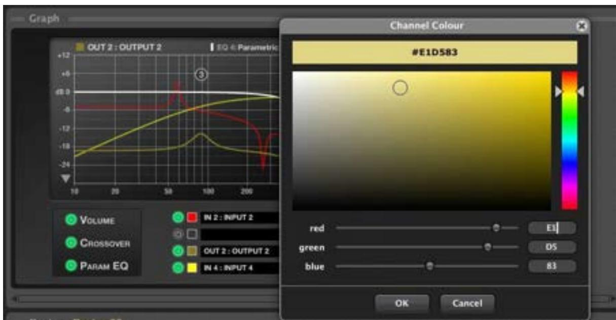
The graph displays the frequency response using a frequency X axis (logarithmic, in Hz) between 10 and 20,000 Hz, and a gain Y axis (in dB) between +12 dB and -30 dB, or between +12 dB and -72 dB (depending on the status of the Vertical Range button, located in the lower left corner of the graph).
