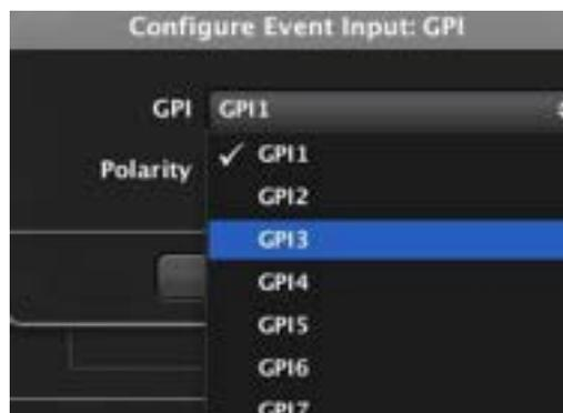
After that, you can define whether the GPI signal will be directly interpreted (0 VDC is considered as the minimum and 10 VDC as the maximum) or inverted (the opposite of the previous case). This setting allows a potentiometer to set a maximum volume in the fully CW position and a minimum volume in the fully CCW position, or vice versa.
