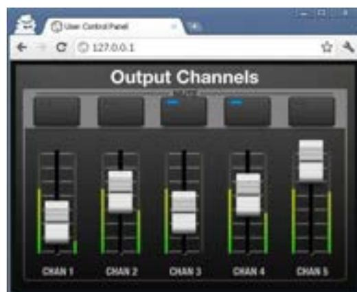
Different web clients can simultaneously load different UCPs and operate the project at the same time, each one controlling a part of the system.
