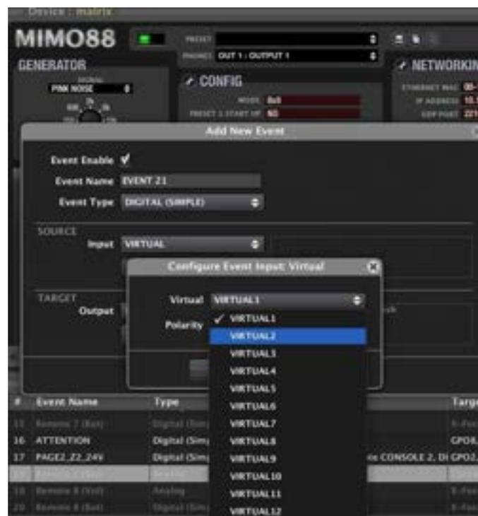
Thus, a UCP button could be used for example to activate a MIMO88's GPO or as a compound digital event input, a type of event that uses Boolean logic operators (AND, OR, NOR, XOR, etc..) to trigger an action depending on the status of various inputs. For example, an event of this type could be "if the GPI #1 of the MIMO88 named OUTDOOR AREAS is closed (AND) a specific UCP button is activated, the *Emergency Preset* should be recalled in this MIMO88 unit".
