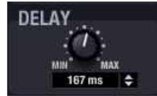
The delay time can be specified in different units, selected with *UNITS* parameter. Available units are milliseconds, seconds, centimetres and meters. *DELAY* can be set between 0 and 1000 milliseconds.
