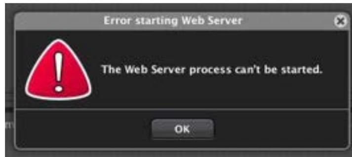
If you click on **OK** EclerNet Manager will run normally, but the web server service is not enabled, making it impossible to connect from client devices and use the project UCPs. Clients will display error messages like this one if you try to connect to the web server:
