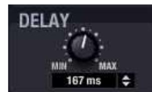
To avoid weird and annoying noises in the output signal, the value change made with the *DELAY* potentiometer is not effective until the mouse button is released. At that time audio will be temporarily muted (for a variable time, depending on the delay value used) for the new setting to be effective.
