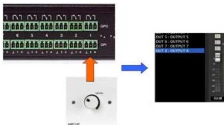
The picture is a representation of a WPMVOL physically connected to the GPI 1 and assigned to the volume of MIMO88's output 8 by EclerNet Manager programming
