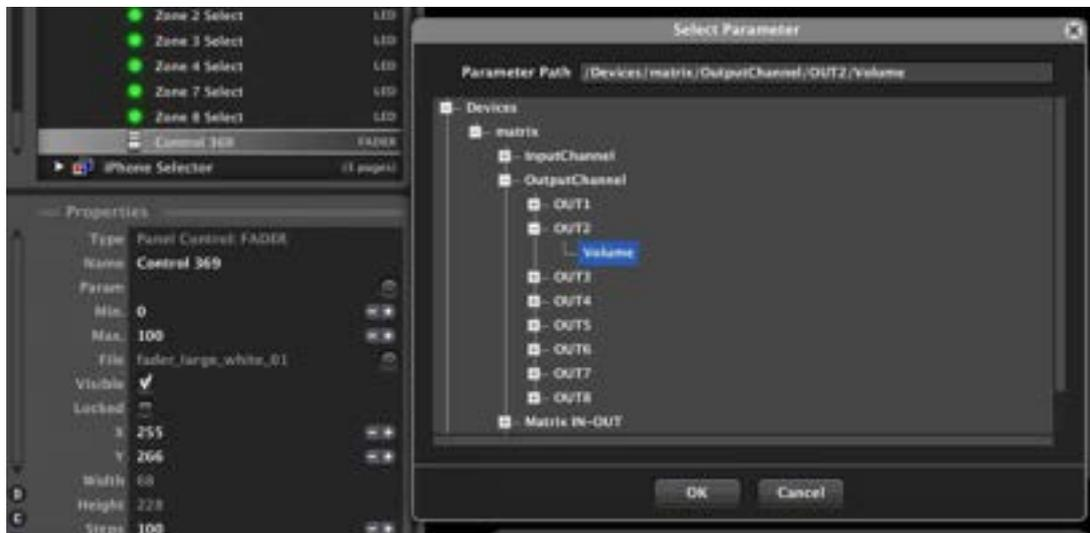
Then a browser window (Select Parameter) opens to select a hardware unit of the project and, within it, a parameter to control. Continuing the example above, the fader that is now displayed with its new appearance (large, white) will control OUT2 volume in a device called "matrix" (in this case a MIMO88).
