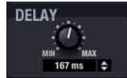
The delay time can be specified in different units, which are determined by the UNITS selector (up and down arrows to the right of the text box). Available units are milliseconds, seconds, centimetres, and meters. DELAY can be set between 0 and 1000 milliseconds.
