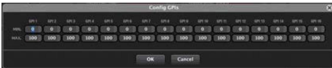
Example for calibrating a WpMVOL / WPaVOL hardware potentiometer connected to GPI #2 to remotely manage a volume control of MIMO88:
