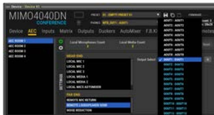
The output can be one of the 8 MIMO4040CDN analogue outputs or one of the 32 Dante™ / AES67 digital outputs. As for the INPUT PORTS, the label can be customized using the “N” button.
