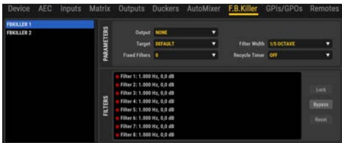
The FEEDBACK KILLER section consists of 2 banks, with 8 automatic filters in each one of them. The 2 banks are independent in terms of settings, operating mode and assigned output.
