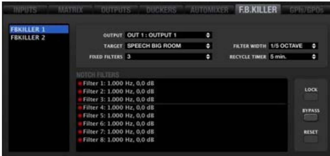
The FEEDBACK KILLER section consists of 2 banks, with 8 automatic filters in each one of them. The 2 banks are independent in terms of settings, operating mode and assigned output.
