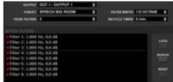
A horizontal line visually separates fixed filters (the first three in this picture) from dynamic filters (the following five in this picture). Dynamic filters can be reset over time if the algorithm detects that it is necessary (microphones moved in the room, changes in the acoustic conditions, etc.).
