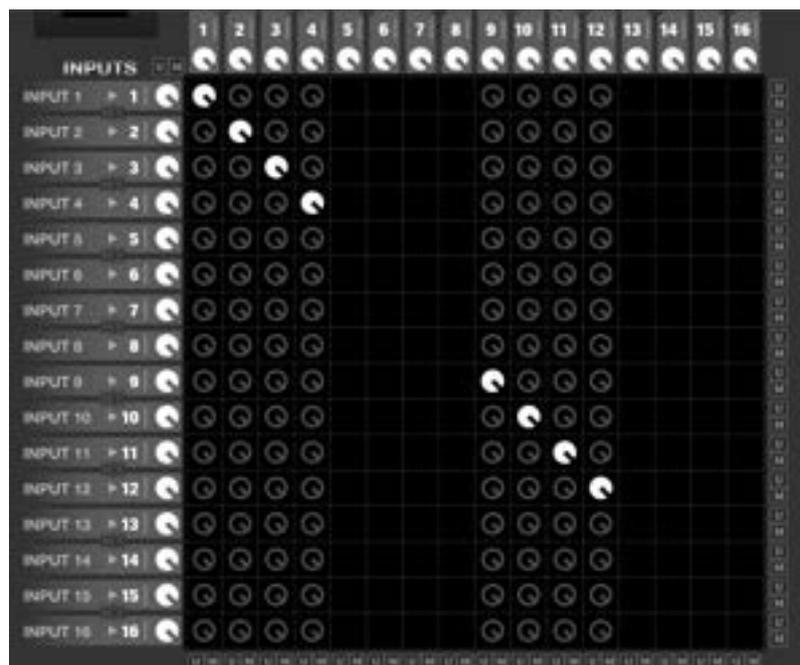
In this case it is possible to process up to 8 independent mixes (outputs 1 to 4 and 9 to 12) using any combination of the 16 available inputs as sound sources.
