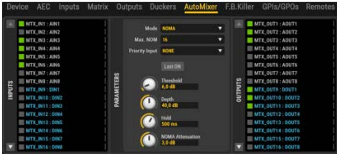
The AUTOMIXER processing module uses a very sophisticated algorithm to manage what input signals must be part of the automatic mix and under what conditions, and what signals must remain apart. The AUTOMIXER analyses the audio content on all inputs to identify what should be considered as background noise and what should be considered as a valid signal to trigger the input channel in the auto mix.
