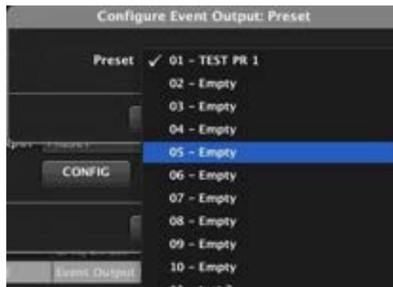
**!** It is important to understand that a **Preset is restored only when there is a rising edge as a stimulus**. In the case of a simple digital event, if it is designed to recall a Preset, you must be sure that there will be a rising edge (0 to 1) as a stimulus, whatever the input type (GPI, UCP button)
