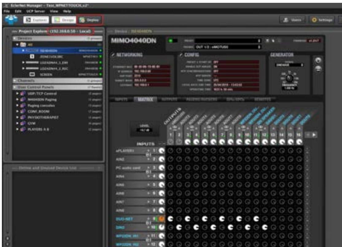
In the above image the Project Explorer window indicates that the project is running in **Local** mode, i.e., in the computer whose IP address is displayed, and not (yet) in a WPNETTOUCH unit. In this state, the computer is acting as a UCP server.
