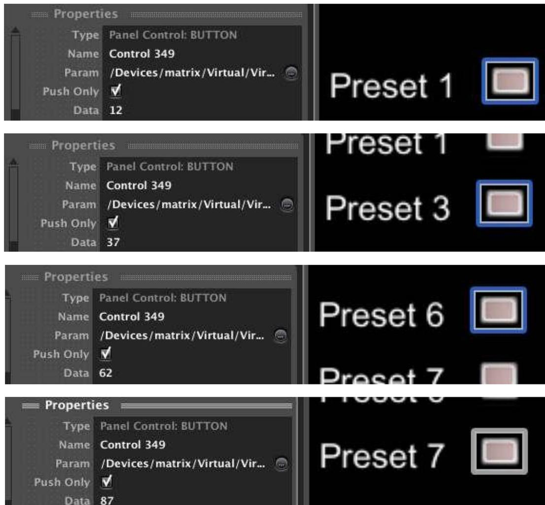
LED indicators can also be associated with virtual controls and you can define the **Data** value such controls should have for the LED to light up.
