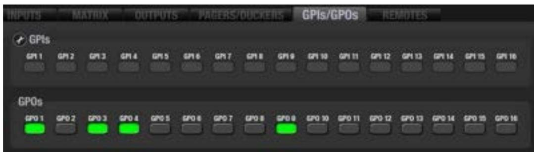
MIMO88's GPI and GPO ports allow you to connect external control hardware and to interact with these units: potentiometers, push buttons, limit switches, lights, motors, etc.
