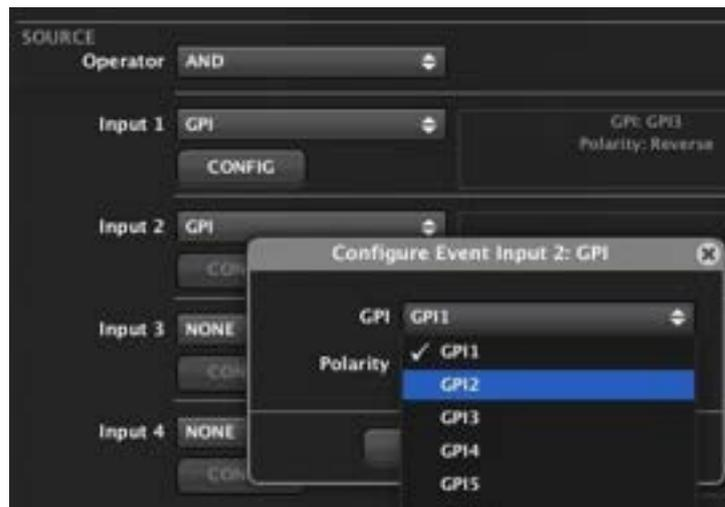
For each of them it's necessary to select the input (GPI, EVENT OUTPUT...) and the DIRECT/REVERSE polarity (0 VDC for 0 and 10 VDC for 1, or vice versa), exactly as for simple digital events. Using EVENT OUTPUT as input for one of the stimuli allows you to concatenate stimuli and thus to exceed the limit of 4 stimuli combined with a logical operator to operate on the same target.
