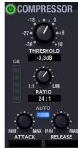
Setting the compressors' *ATTACK* and *RELEASE* times correctly is not an easy task: too short release or attack times result in excessive and perceptible low frequencies distortion; on the other hand, too long times could make a limiter useless if damages already occurred before limitation starts.
