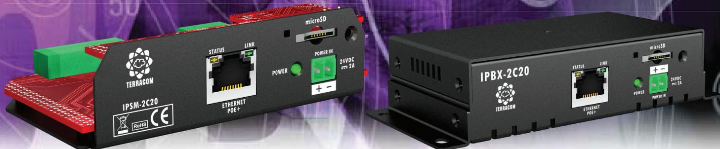
The IPISM-2C20 and IPBX-2C20 speaker modules are equipped with 2x20w audio channels and an 8ohm loudspeaker output that can also be bridged to a single 40w/4ohm channel. While supporting PoE+ (power over ethernet), an external power adapter can also be provided to supply further power (24VDC). PoE+ offers a cost-effective solution for paging, audio challenges, intercom, and background music systems over a standard RJ45 ethernet connection by minimising the number of cables required.
