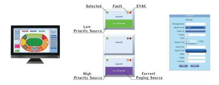
To create and expand the paging zones in TerraManager, the BOUTIQUE system can be integrated with TerraManager via LAN/WAN for network paging and intercom control. The TerraManager will control/monitor the BOUTIQUE controller and the connected Terracom device will act as an "agent".
