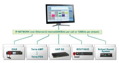
The TerraManager is an integrated control software which operates on a touch screen PC/Laptop and provides an GUI components to control ATEIS products such as IDA8, BOUTQIUE, and TERRACOM system etc., and can also support by 3rd party control.
