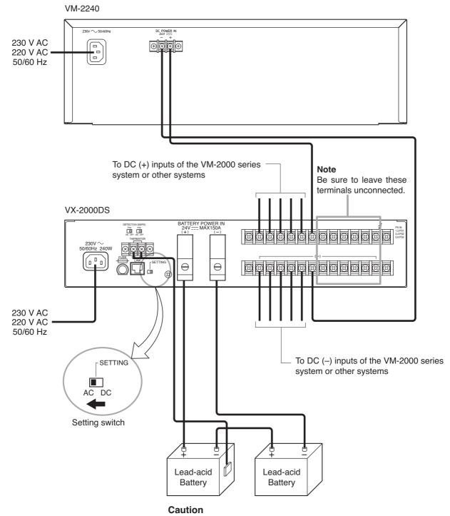
The charging current from VX-2000DS is 5 A maximum. Applicable Batteries: Panasonic LC-X1265PG/APG
