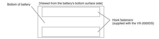
When replacing the batteries, 4 each of fastener hooks and loops, and a thermal insulating sheet listed below are also required. Consult your nearest TOA dealer on how you can obtain them.
