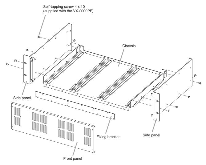
Note: Mount the front panel and fixing bracket after installing the VX-200PS units on the chassis.
