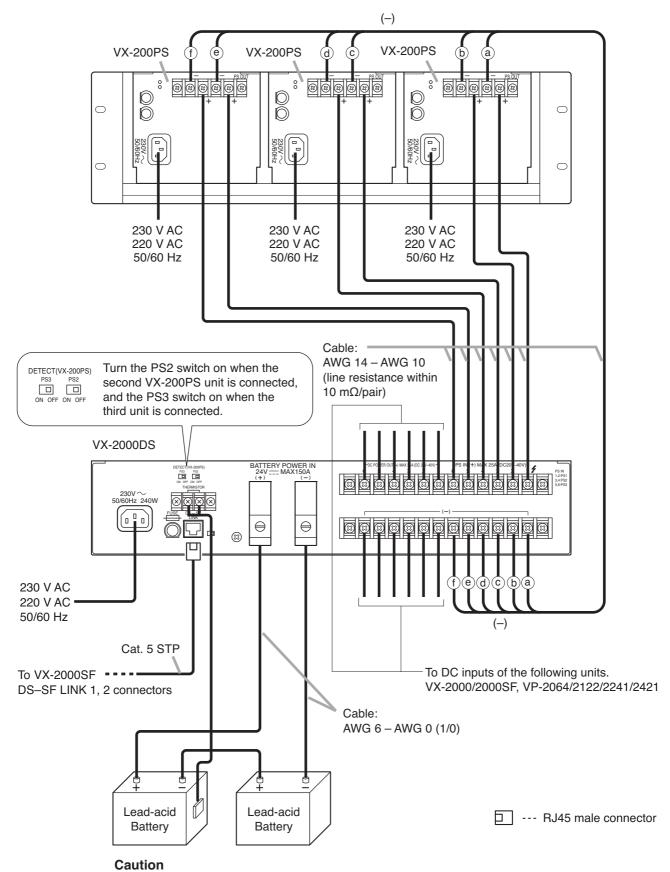
The charging current from VX-2000DS is 5 A maximum. Applicable Batteries: Panasonic LC-X1265PG/APG
