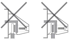
Strip the cable end long enough (30 mm ± 5 mm) to be fully clamped. Otherwise, its outer jacket prevents the cable conductor from being tightly secured, causing poor contact.
