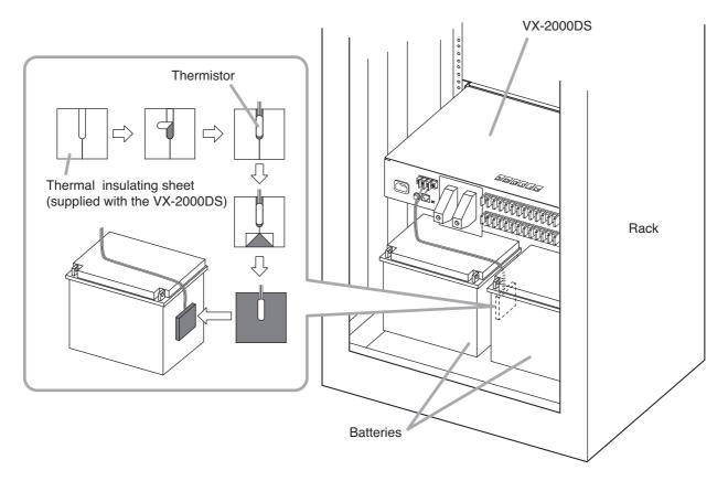
Step 1. Clean the exterior surface of the battery using a soft damp cloth.
