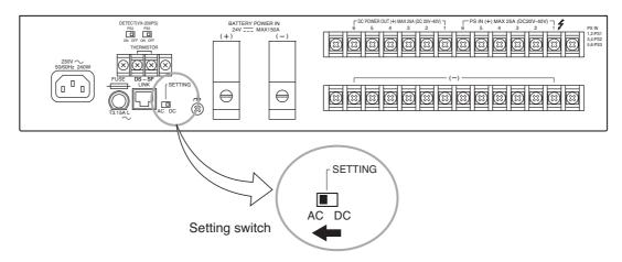
Step 3. Stop the AC power supply to the VX-200PS.
