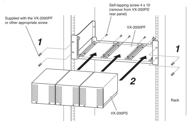
Step 3. Fit the VX-2000PF's fixing bracket and front panel in place.
